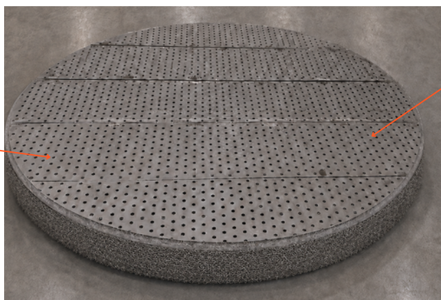
The pressure equalization plate and demister pad
