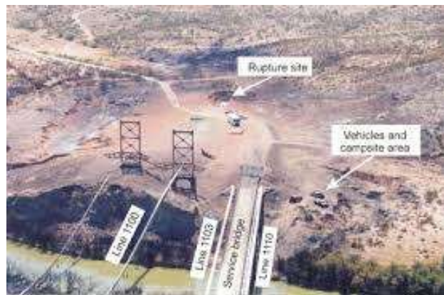
Figure 13. Rupture site showing crater and bridge supports
