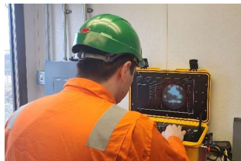
Figure 2. A live view from inside a high pressure gas pipeline
