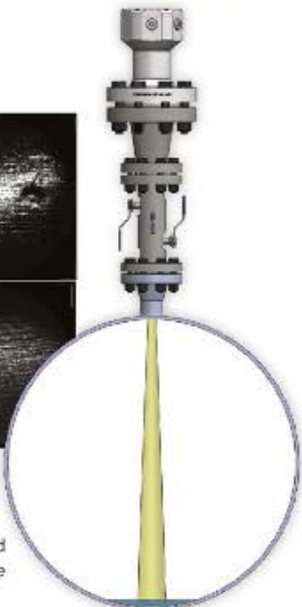
LineVu mounted on a gas pipeline
