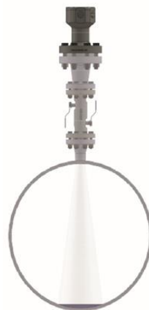
Figure 19. LineVu system mounted on top of a pipeline
