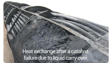
Heat exchange after a catalyst failure due to liquid carry-over.
